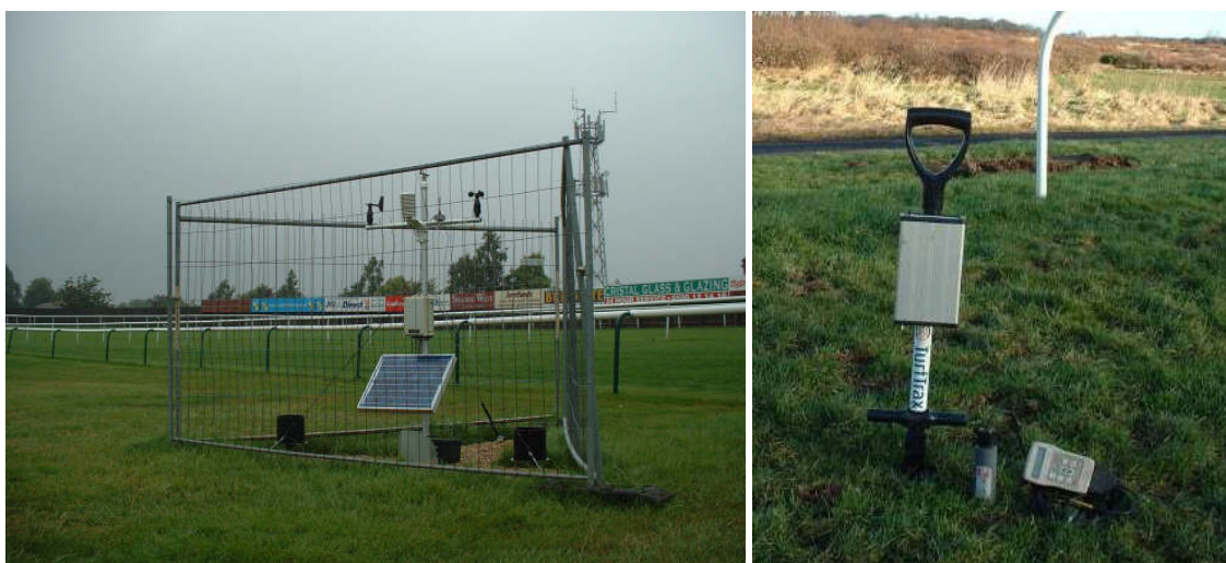
Figure 5 An on-course weather station (left) and theta probe inserted next to GoingStick (right)
